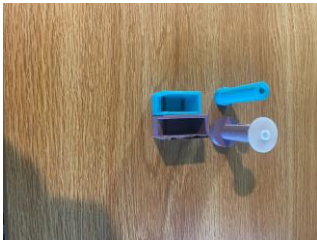
Figure 117. 3D Printed Servo Motor Holders and Dowels (First design on left and final design on right)
