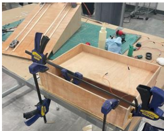
Figure 67. Upside-Down Combined Keyboard Cover and Button Board During Construction
